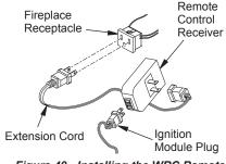
Figure 40 - Installing the WRC Remote Receiver
